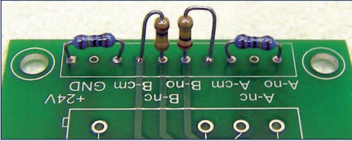
*Figure 2: Image of ALD coated through hole components soldered to a board with the solder wetting up to the coated area. Image courtesy of Sundew Technologies, LLC.*
