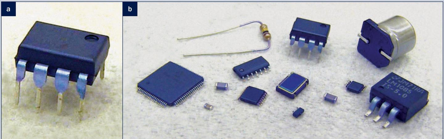
Figure 1: Images of ALD coated components with the solderable surface left uncoated. The ALD coating has a matte appearance while the uncoated region appears glossy. Image courtesy of Sundew Technologies, LLC.
