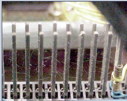
*Figure 1: Pure tin plated connector pins displaying many short circuits due to tin whisker growth. Connector was approximately 10 years old. Photo courtesy of NASA.*
