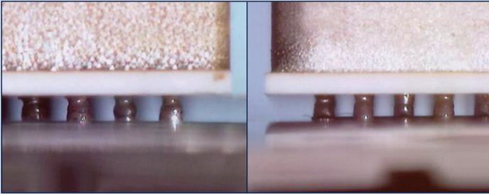
*Figure 2: Coplanarity – High melt joints with .014 inch/inch board warp.*
