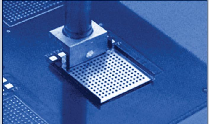
*Figure 3: Ball Grid Array Stencil*
