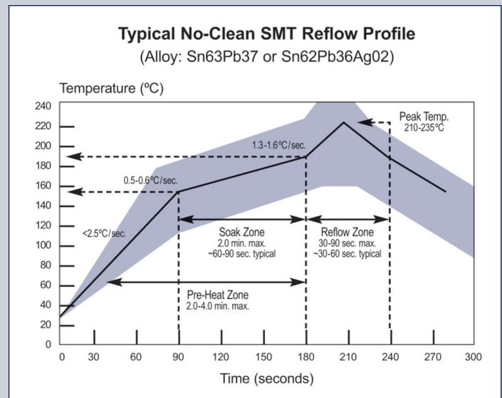
Figure 1: Typical No-Clean SMT Reflow Profile
