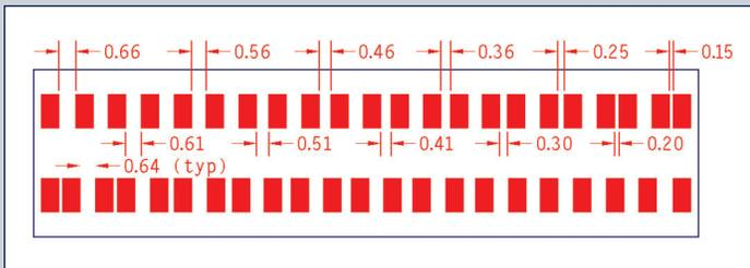
Figure 1: Wetting Test Pattern (dimensions in mm)
