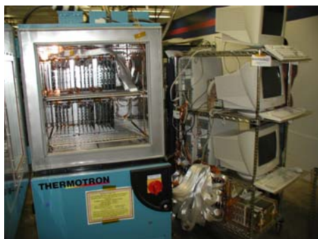
Test Vehicles in the Thermal Cycle Chamber (Rockwell Collins, Cedar Rapids, Iowa)
