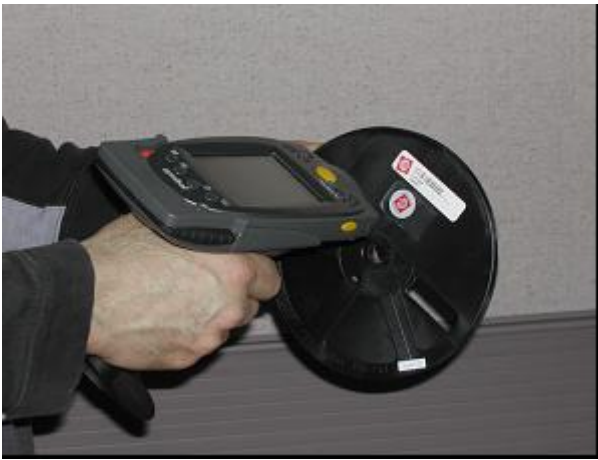
Manual Scanning of Barcode Label
