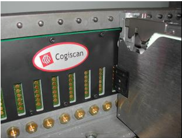
RFID Smart Feeders on placement machine
